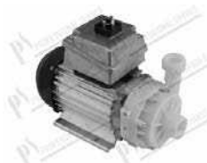
Wash pump 1 phase 290W 220/240V 60Hz inlet Ø 32 mm; outlet Ø 1"
