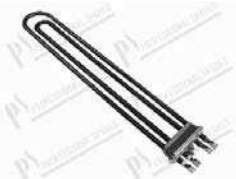
Boiler heating element 6100W 254V dim. 80x460 mm; faston 6.3x0.8 mm
