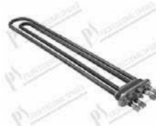
Boiler heating element 6540W 240V L=415 mm; flange 81x28 mm; faston 6,3 mm; with gasket
