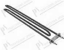
Tank heating element 1220W 254V dim. 420x64x50 mm; flange 81x28 mm; connection M4
