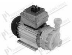
Wash pump 1 phase 240W 220/240V 1,0A 50/60Hz inlet Ø 32 mm; outlet Ø 1"; C=5µF 400V
