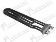
Boiler heating element 6000W 240V dim. 82x350 mm; faston 6.3x0.8 mm
