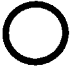
Flat gasket Ø 90x107x2,5 mm
