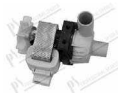
Drain pump 80W 220-240V 50Hz inlet Ø 24 mm; outlet Ø 24 mm; faston P5
