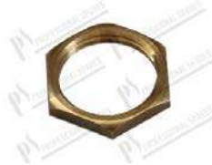
Hexagonal nut 3/4" - H=4,5 mm CH30 mm
